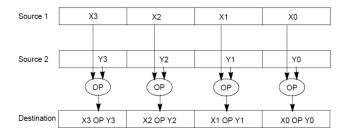
Some machines with x86 architectures have special, wider registers, that can hold 128, 256, or even 512 bits. Intel intrinsics (Intel proprietary technology) allow us to use these wider registers to harness the power of DLP in C code.
