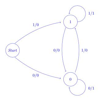
2.3 Draw an FSM that will output a 1 if it recognizes the regex pattern {10+1}. (That is, if the input forms a pattern of a 1, followed by one or more 0s, followed by a 1.)
